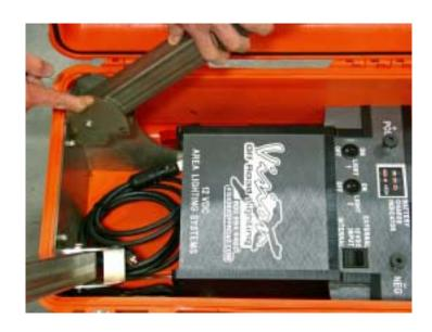
3. The leg can be further extended by pulling out on the leg until it locks. To retract, push in on the pins, both sides, and slide back into its sleeve.
