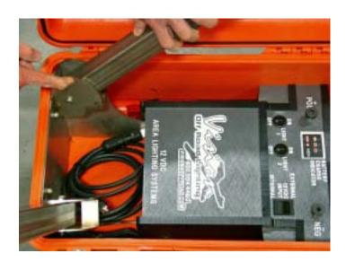
2. Fold light assembly into case by pulling up on mast lock mechanism. Align all thumb screws so that they lay flat against the battery pack. Make sure lights are facing up with the rounded portion of the mast facing out. Close and lock lid.
