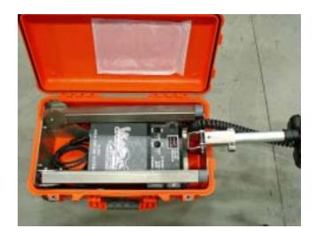
2. To release the stainless steel legs, push in on the pin located at the base of the leg and rotate out until it locks into place.
