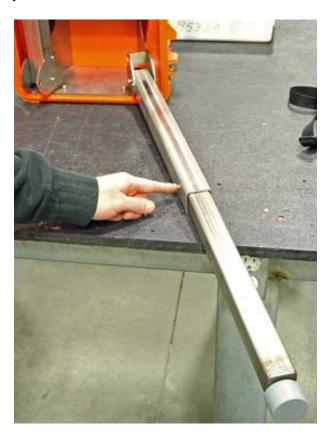
4. Stand the light unit upright and extend the light pole to the desired height. Start with the top thumb screw, extend the pole and tighten into position.
